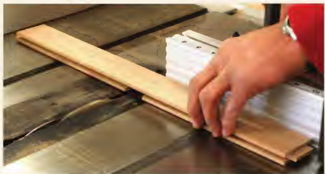
Two stops set the width. The half-lap joint is formed by repeated passes over the table saw blade.
